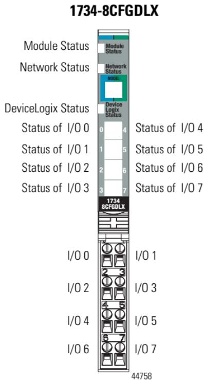
Note that voltage and current to the module is applied through the adapter, the 1734-FPD module, or the 1734-EP24DC module. V = 10...28.8 V DC.
