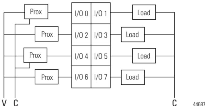
If a connection to Common or the Supply Voltage is required for two- or three-wire devices, then a 1734-CTM or 1734-VTM can be used.
